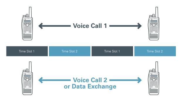
TDMA divides a 12.5 kHz channel into two alternating time slots to achieve 6.25 kHz equivalent spectral efficiency when used with a repeater.
